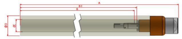
Immersion tubes are made from high density convolute wound paper for maximum strength and resilience. Probes with immersion tubes are available in a variety of lengths.
