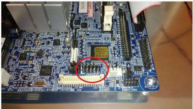
There are 2 rows of pins on the F\_PANEL connector. The bottom row has 5 pins and the top row has 4. You are interested in the top row, two pins to the right. These are pins 6 and 8 which are *Power* and *Ground*.
